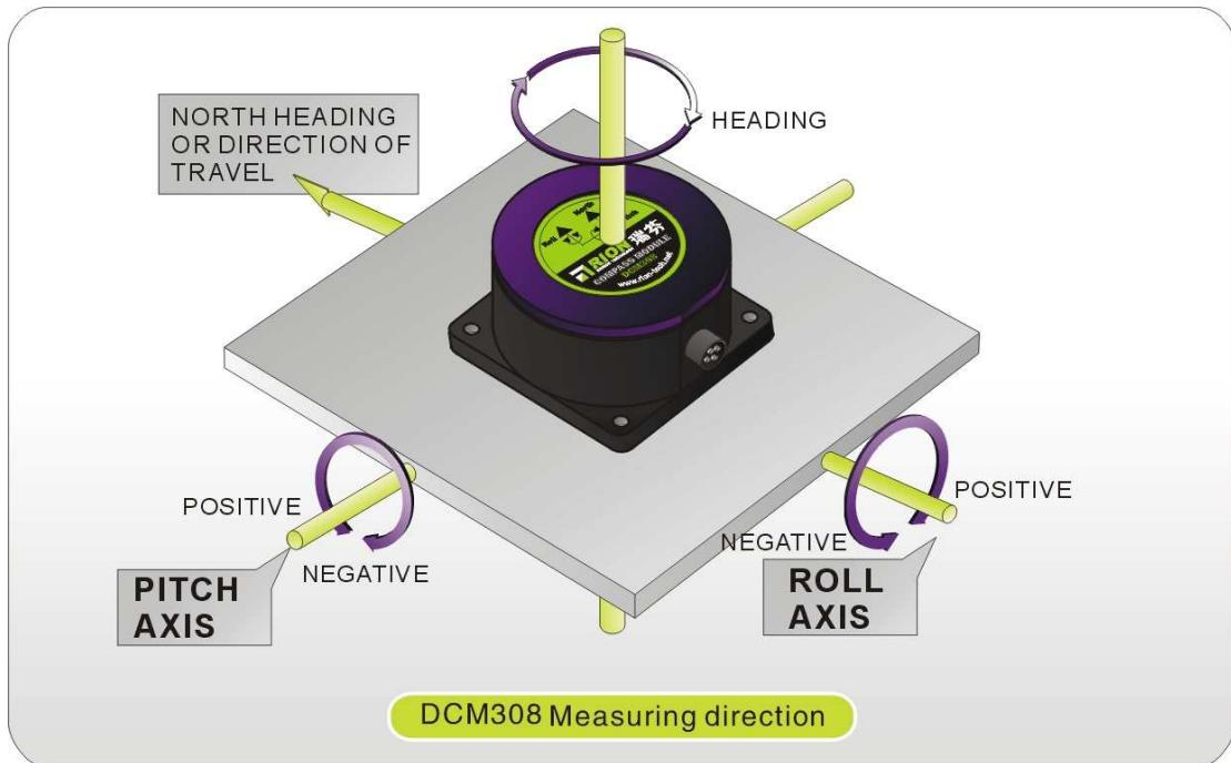
The DCM308's magnetometers' wide dynamic range and its sophisticated calibration algorithms allow it to operate in many environments. For optimal performance however, you should mount the DCM308 with the following considerations in mind:
